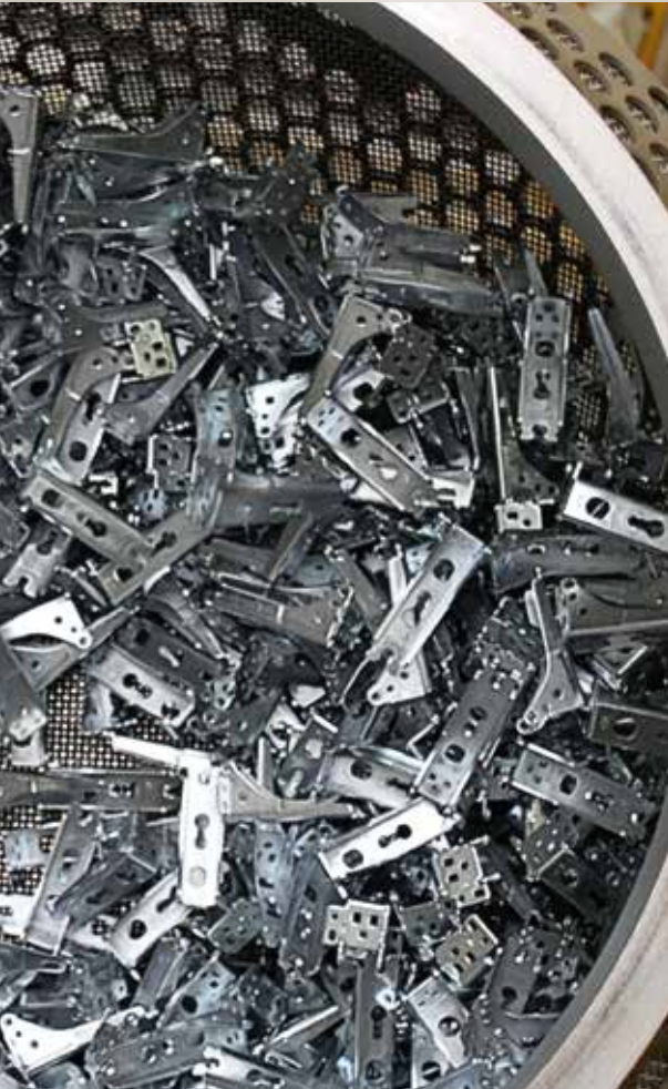
Hinges for the furniture industry, galvanised without using Chromium VI
