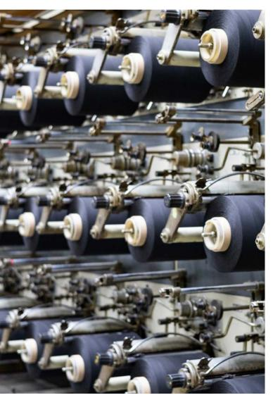
Winding of treated cords in the thread stretching unit.
